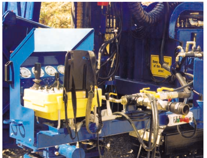
control panel "remote control" / Steuerstand
